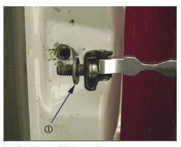
3. Position the check link bracket to the B pillar and reinstall the bolt.
