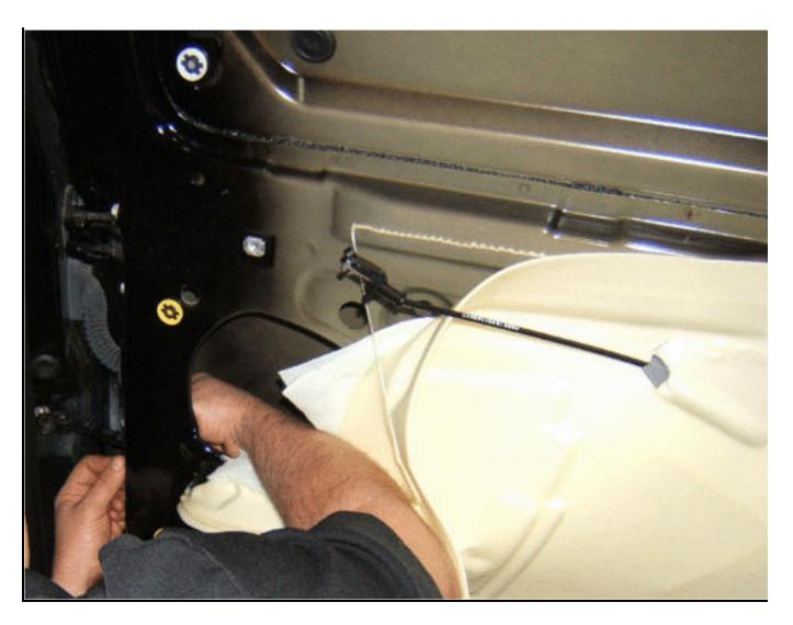
9. Add a 2 mm thick washer (1), P/N 11609679, or equivalent, to each bolt on the check link (two total). Slide them onward to rest against the body of the check link.
