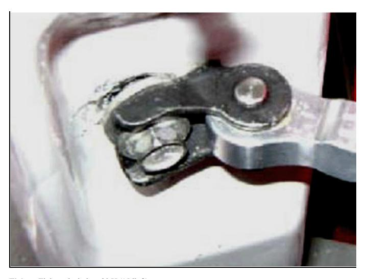
**Tighten** Tighten the bolt to 20 Y (15 lb ft).
