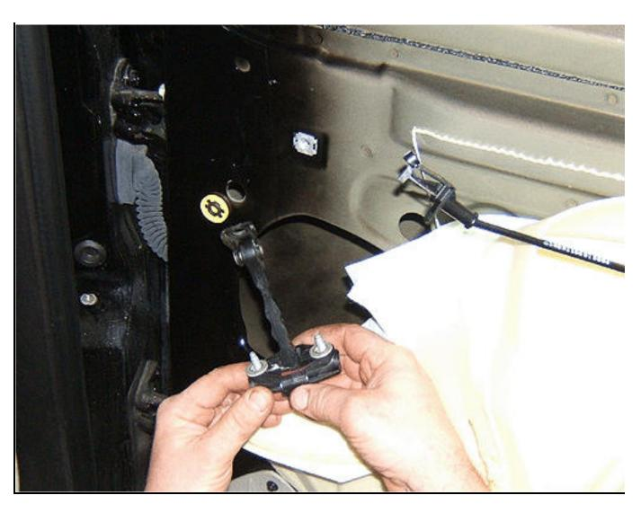
11. Install the nuts (2) that retain the check link to the door.
