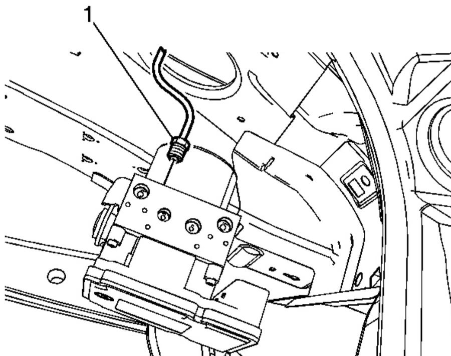
**Fig. 24: LR Brake Pipe Fitting**
