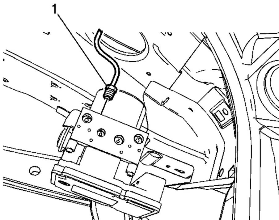
**Fig. 10: LR Brake Pipe Fitting**
