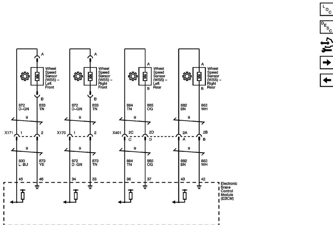
**Fig. 2: Wheel Speed Signals**
