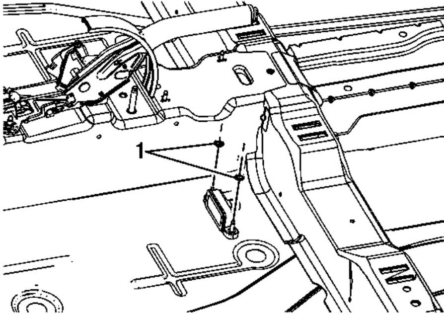
**Fig. 38: View Of Yaw Rate Sensor & Nuts**
