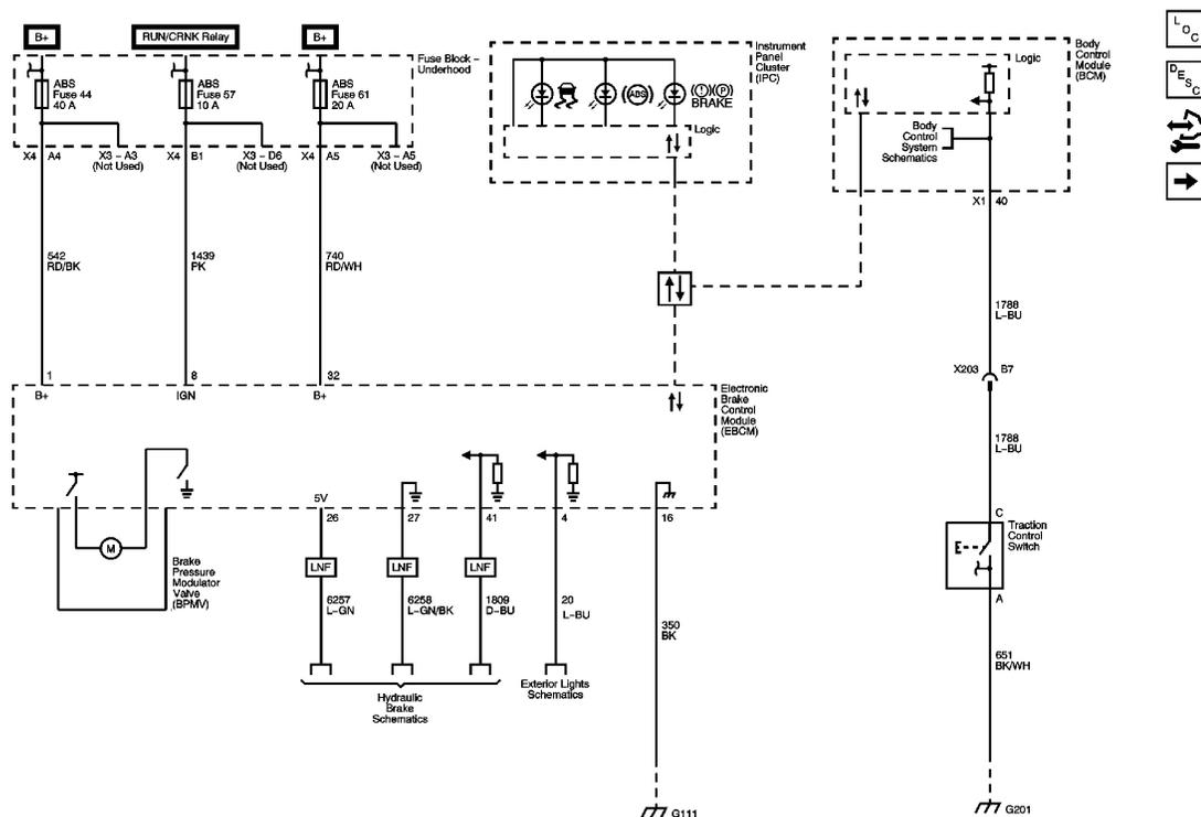
**Fig. 1: Power, Ground, Serial Data and Traction Control**
