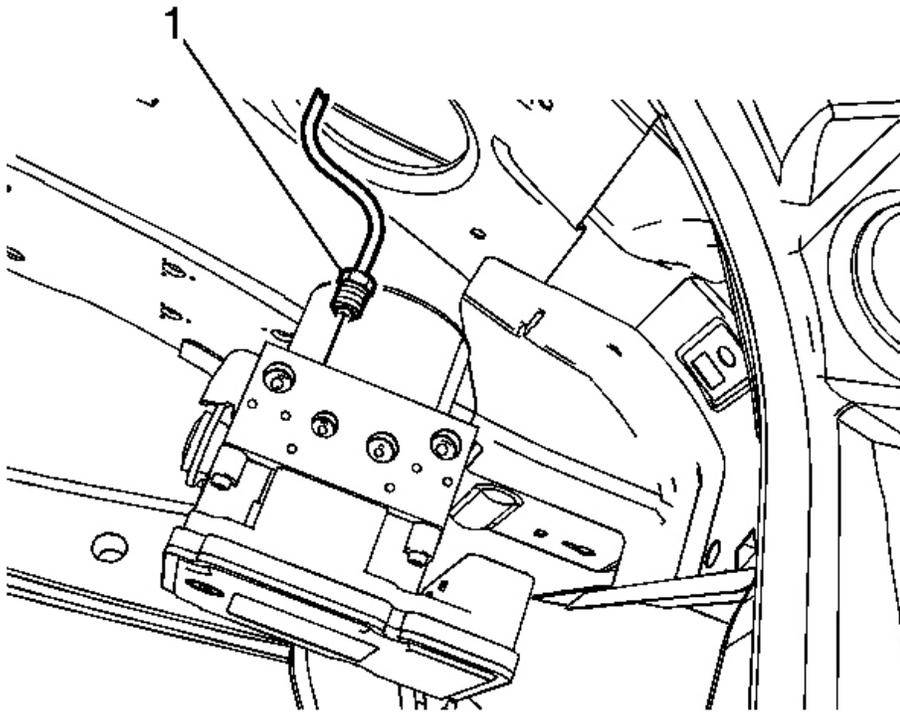
**Fig. 13: LR Brake Pipe Fitting**
