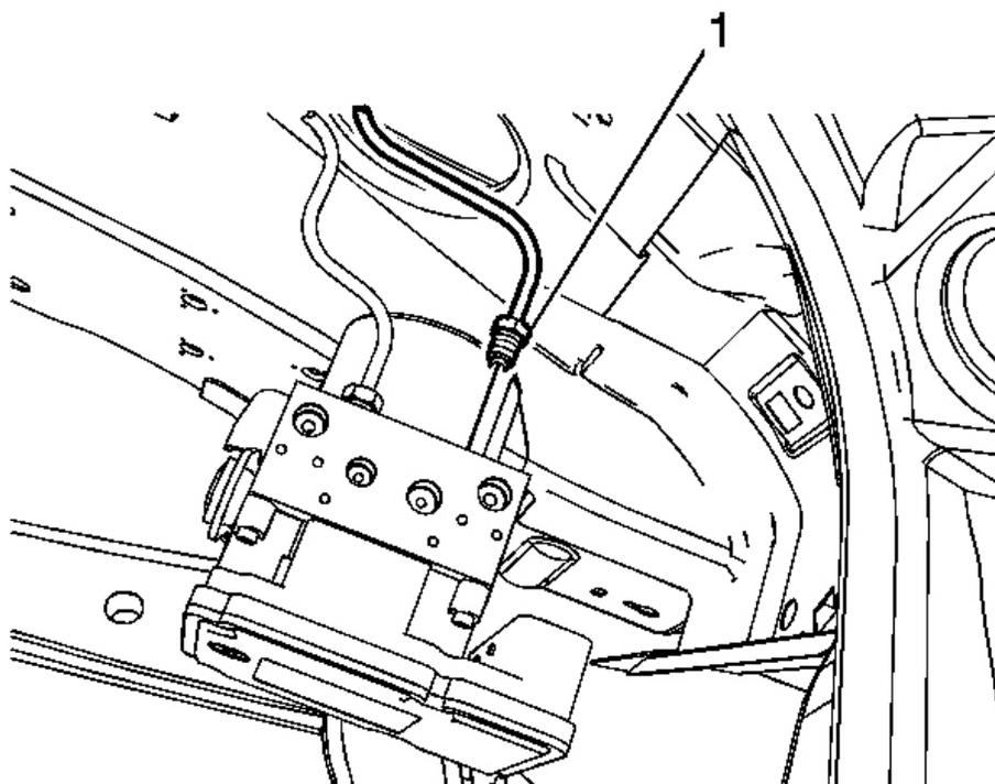
**Fig. 9: RR Brake Pipe Fitting**
