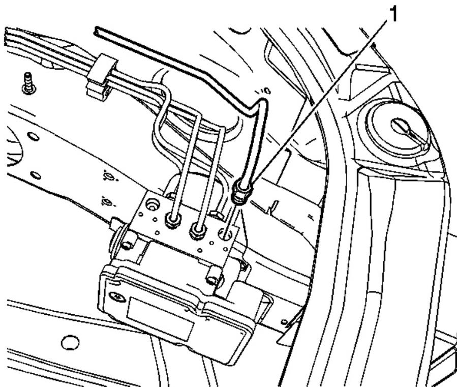
**Fig. 31: Master Cylinder Secondary Brake Pipe Fitting**
