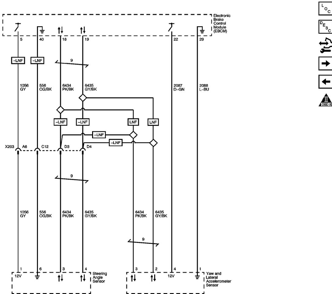
**Fig. 3: Vehicle Stability Control**
