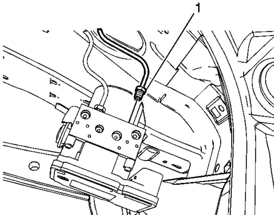
**Fig. 14: RR Brake Pipe Fitting**
