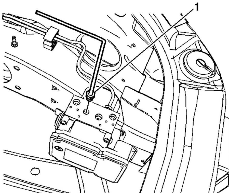
**Fig. 22: RF Brake Pipe Fitting**
