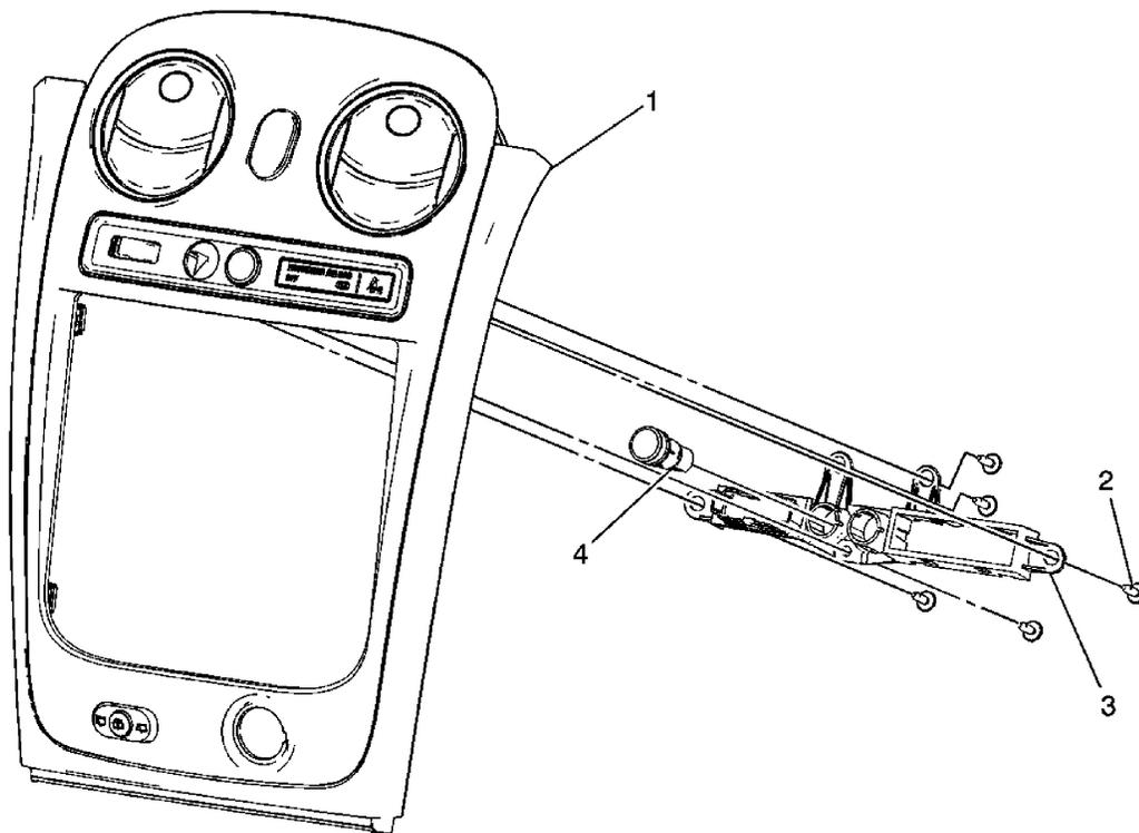
**Fig. 37: Electronic Traction Control Switch**
