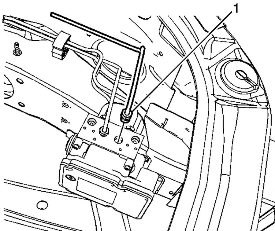
**Fig. 16: LF Brake Pipe Fitting**
