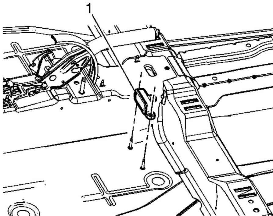
**Fig. 39: View Of Yaw Rate Sensor**
