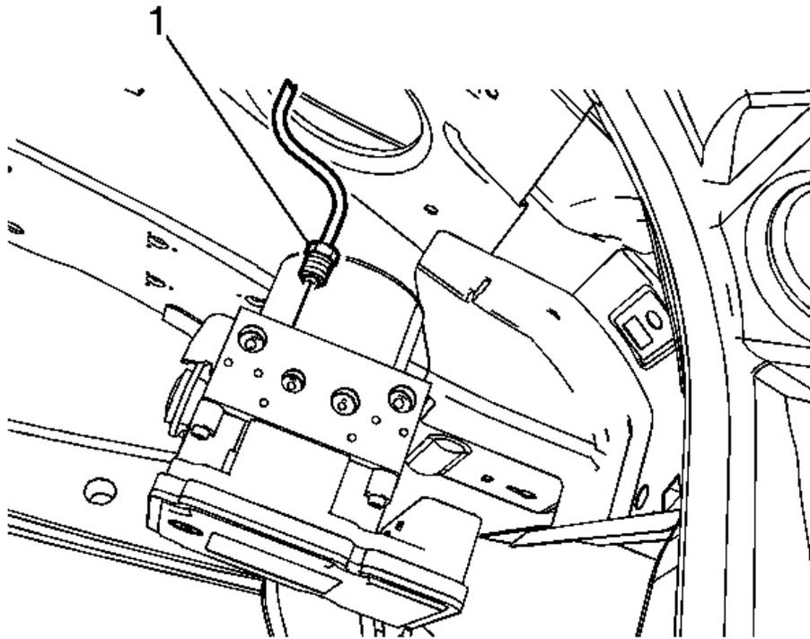
**Fig. 27: LR Brake Pipe Fitting**
