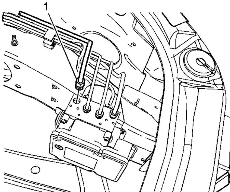
**Fig. 19: Master Cylinder Primary Brake Pipe Fitting**
