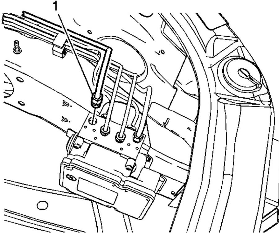
**Fig. 18: Master Cylinder Primary Brake Pipe Fitting**
