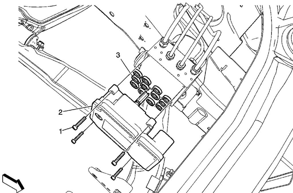
**Fig. 4: Electronic Brake Control Module (With JL4)**
