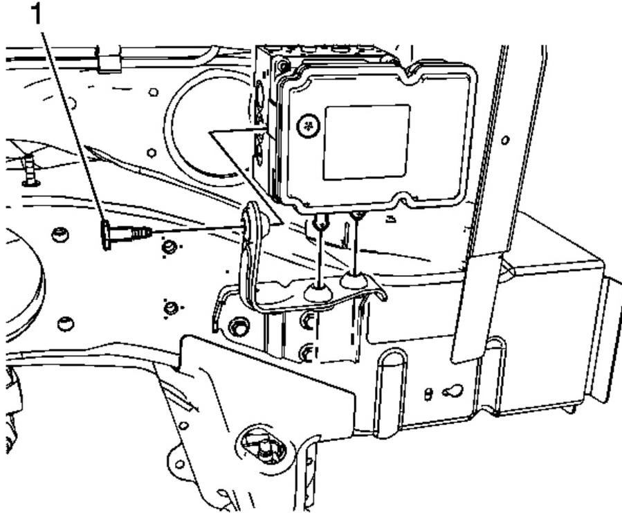
**Fig. 33: Brake Pressure Modulator Valve (BPMV) Bolt**
