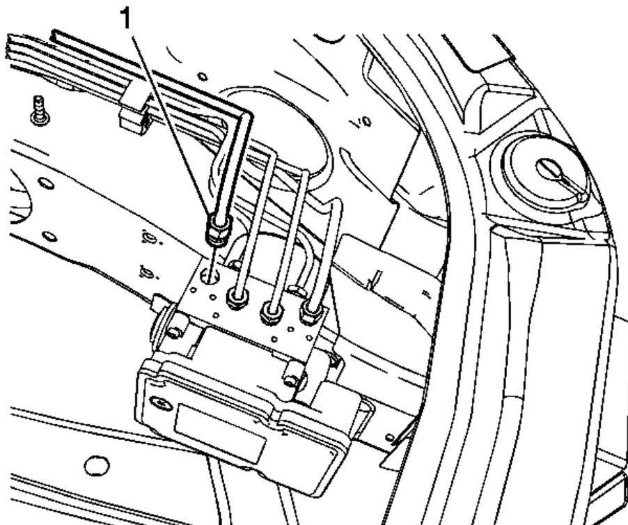
**Fig. 32: Master Cylinder Primary Brake Pipe Fitting**
