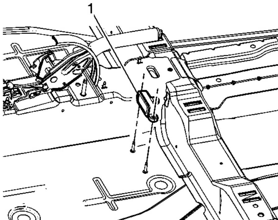
**Fig. 40: View Of Yaw Rate Sensor**
