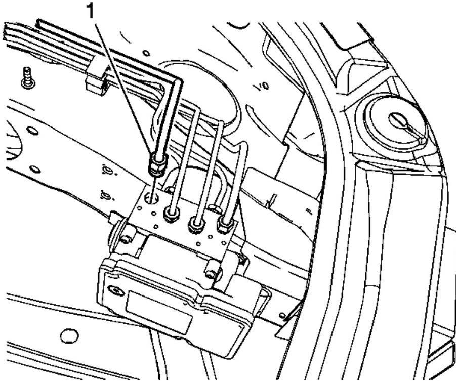
**Fig. 5: Master Cylinder Primary Brake Pipe Fitting**
