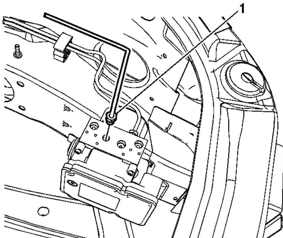
**Fig. 15: RF Brake Pipe Fitting**
