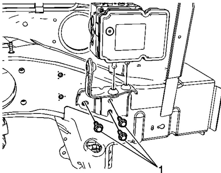
**Fig. 35: Upper BPMV Bracket Bolts**
