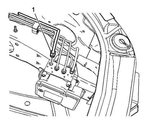
Fig. 19: Master Cylinder Primary Brake Pipe Fitting Courtesy of GENERAL MOTORS CORP.
