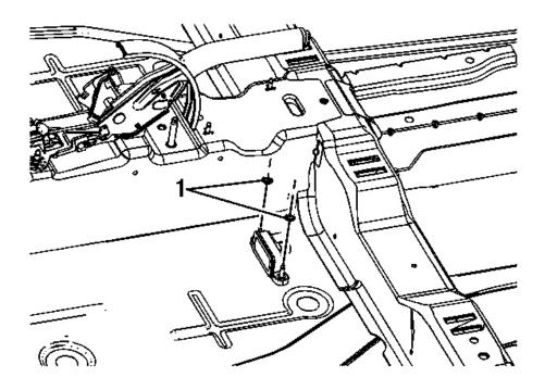
Fig. 38: View Of Yaw Rate Sensor & Nuts Courtesy of GENERAL MOTORS CORP.
