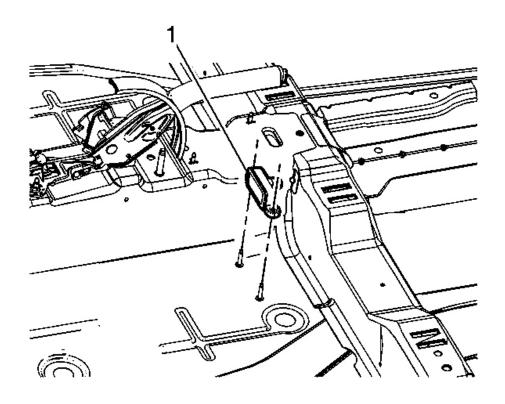
Fig. 40: View Of Yaw Rate Sensor Courtesy of GENERAL MOTORS CORP.
