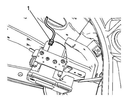
Fig. 24: LR Brake Pipe Fitting Courtesy of GENERAL MOTORS CORP.
