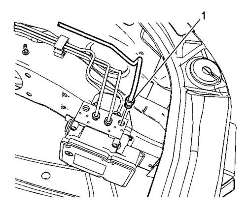
Fig. 6: Master Cylinder Secondary Brake Pipe Fitting Courtesy of GENERAL MOTORS CORP.
