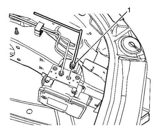
Fig. 21: LF Brake Pipe Fitting Courtesy of GENERAL MOTORS CORP.
