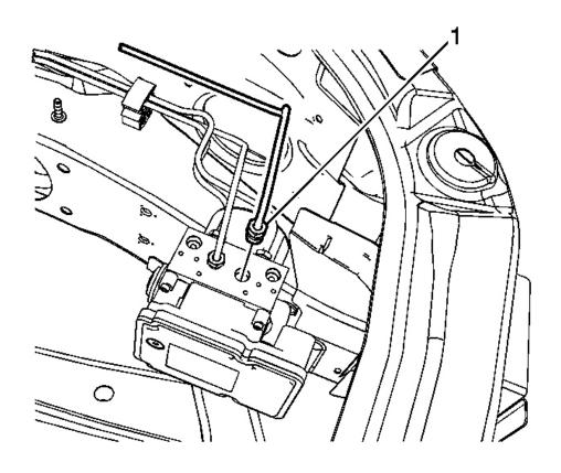
Fig. 7: LF Brake Pipe Fitting Courtesy of GENERAL MOTORS CORP.
