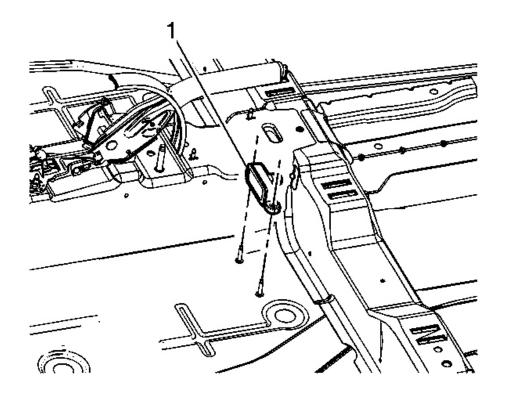
Fig. 39: View Of Yaw Rate Sensor Courtesy of GENERAL MOTORS CORP.
