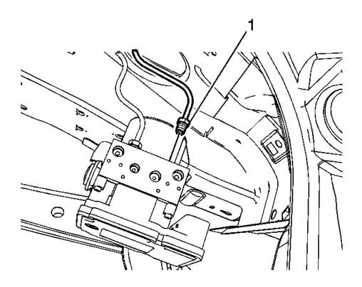
Fig. 9: RR Brake Pipe Fitting Courtesy of GENERAL MOTORS CORP.
