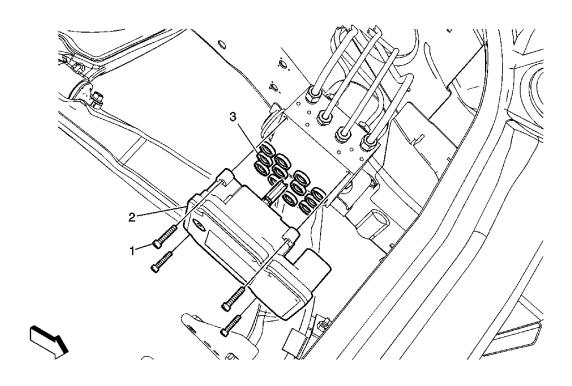
Fig. 4: Electronic Brake Control Module (With JL4) Courtesy of GENERAL MOTORS CORP.
