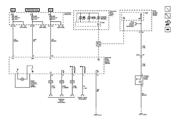
2010 BRAKES Antilock Brake System - HHR
