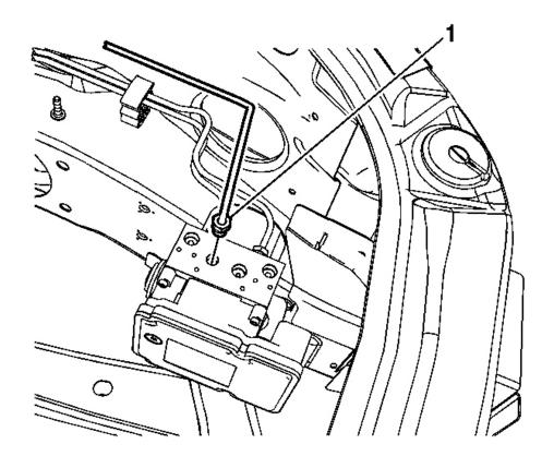
Fig. 29: RF Brake Pipe Fitting Courtesy of GENERAL MOTORS CORP.
