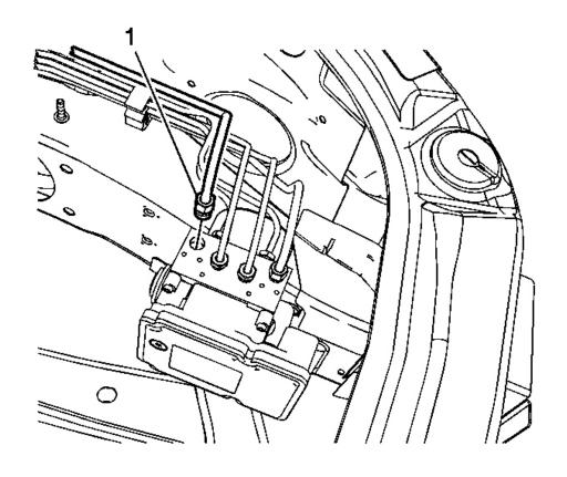
Fig. 32: Master Cylinder Primary Brake Pipe Fitting Courtesy of GENERAL MOTORS CORP.
