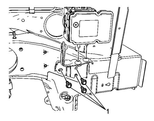
Fig. 34: Upper BPMV Bracket Bolts
