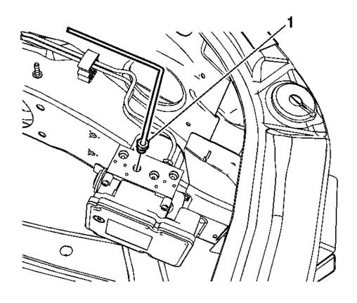
Fig. 8: RF Brake Pipe Fitting Courtesy of GENERAL MOTORS CORP.
