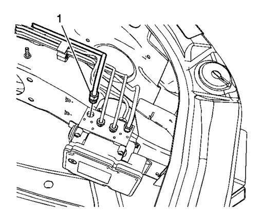
Fig. 18: Master Cylinder Primary Brake Pipe Fitting Courtesy of GENERAL MOTORS CORP.
