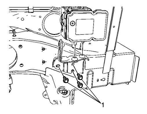
Fig. 35: Upper BPMV Bracket Bolts
