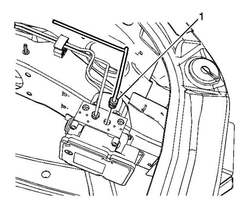
Fig. 30: LF Brake Pipe Fitting Courtesy of GENERAL MOTORS CORP.
