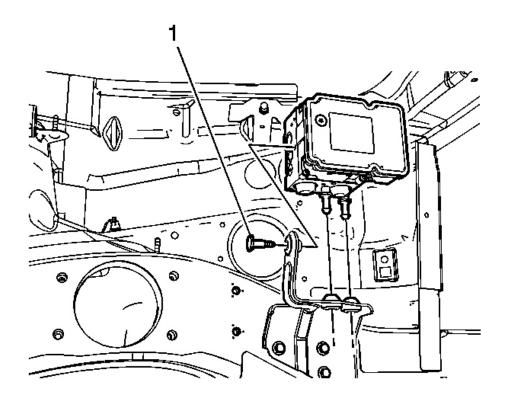
Fig. 12: BPMV Bolt Courtesy of GENERAL MOTORS CORP.
