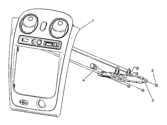
Fig. 37: Electronic Traction Control Switch Courtesy of GENERAL MOTORS CORP.
