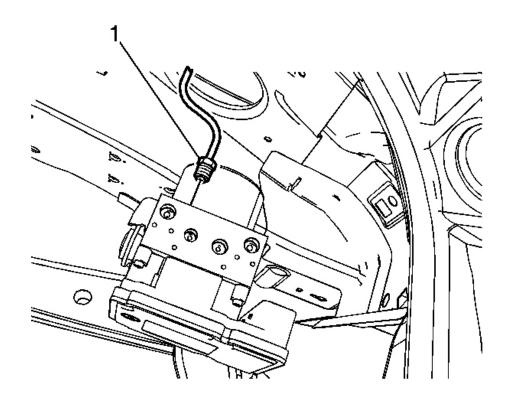
Fig. 10: LR Brake Pipe Fitting Courtesy of GENERAL MOTORS CORP.
