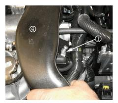
3. Remove the CAC duct (4) off of the first design mounting stud (1).
