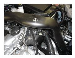
2. Locate the charge air cooler (CAC) duct (4).
