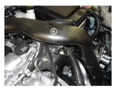
6. Secure the CAC duct (4) onto the second design mounting stud.
